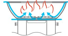
The fire is fed from below and around the side of the bowl. Air flows up through the fire grate to keep your fire burning strong.
