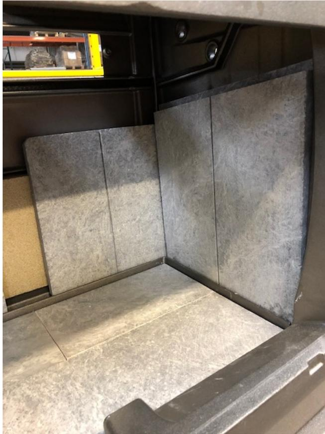
**Photo 4. Right side refractory stone installed.**
