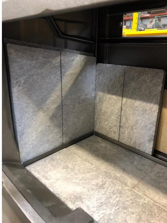
**Photo 2. Left side refractory stone installed.**
