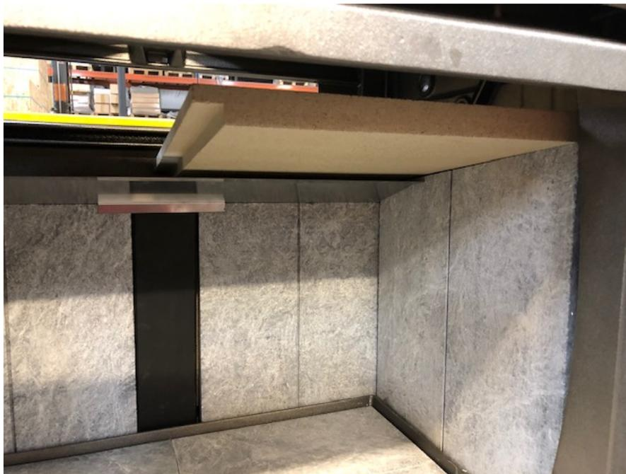
**Photo 6. Right side baffle half installed.**
